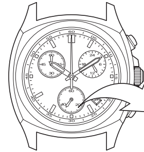
[Insufficient Charging Warning Feature] The second hand switches from 1-second interval movement to 2-second interval movement
